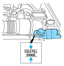
If the engine coolant has not been checked at the recommended interval, the engine coolant reservoir may become empty. If this occurs, add engine coolant to the reservoir. For more information on engine coolant maintenance, refer to *Adding engine coolant* in this chapter.
